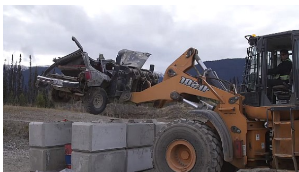
Figure 3. Placing ELV on cinderblocks
