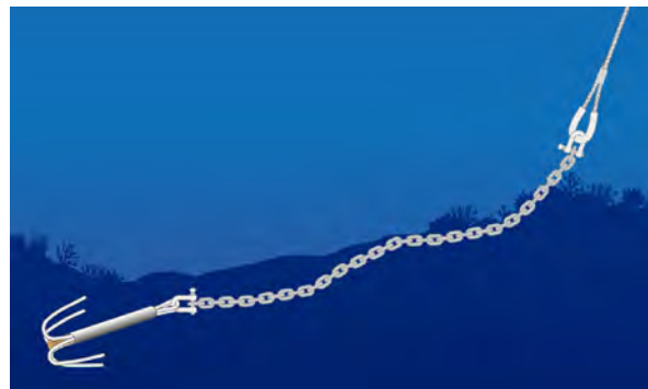
A short length of chain prevents the rope from chafing on the sea floor.
