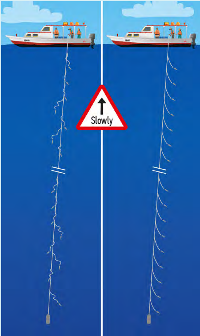
If the vertical longline is hauled in too fast (left), branchlines will tend to wrap around the mainline.
