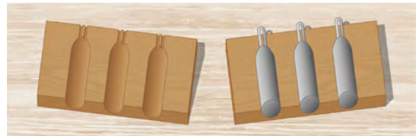
...or you can make your own from wood, or even cardboard set in a bed of sand.
