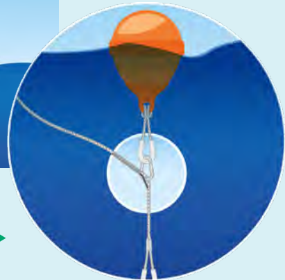
The non-return barb prevents the chain and anchor from sinking back to the bottom.
