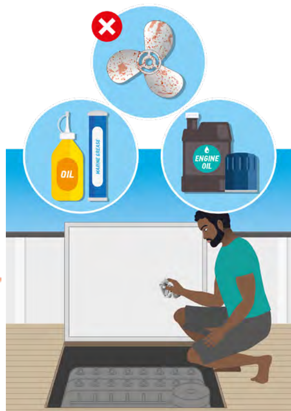
Wipe the engine with a clean rag and fresh water, check the engine and gearbox oil.
