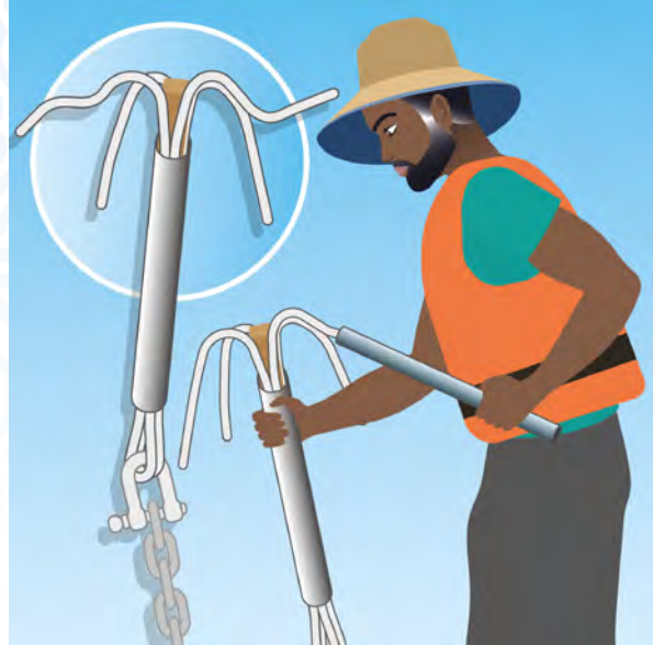
Using a length of steel pipe helps to bend the prong back to the correct shape.
