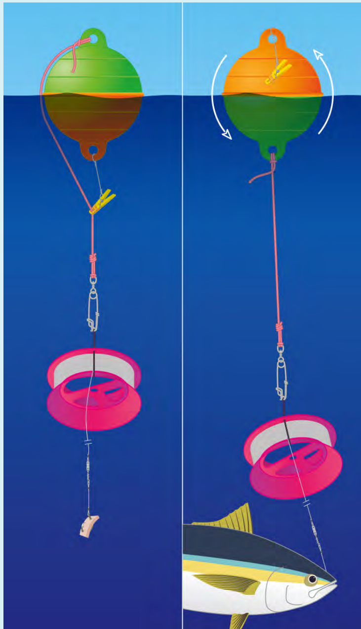
When a fish strikes, the clip releases the braided cord, and the orange side of the float turns upwards, indicating a fish is hooked.
