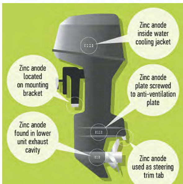
Some outboard motors carry multiple anodes.
