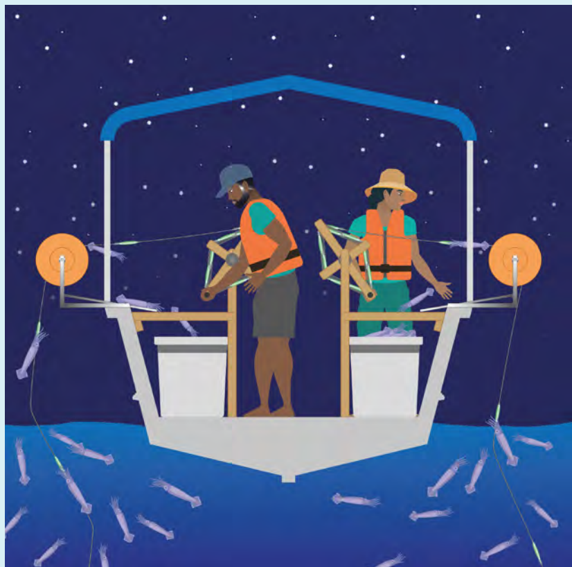
Small boat squid jigging setup, using modified FAO wooden hand reels and wide rollers.
