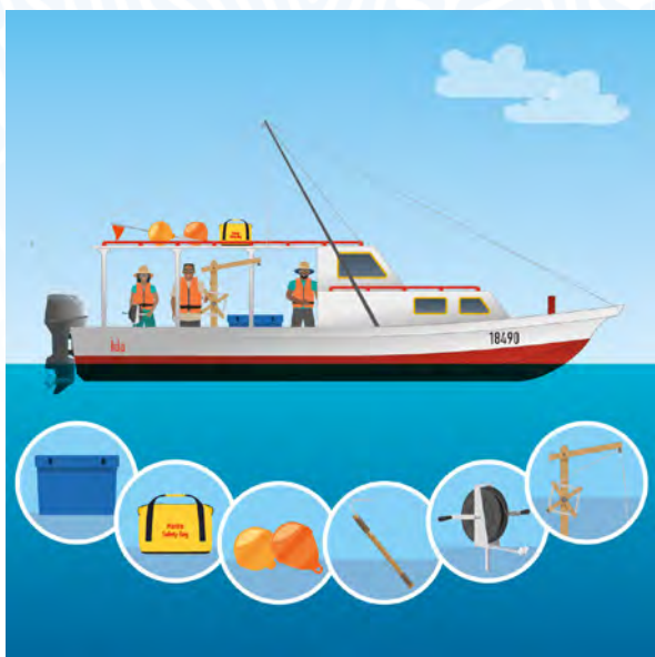
Cabin boat equipped for nearshore trolling, mid-water and deep-bottom fishing. Equipment includes a large icebox, a safety grab bag, a couple of floats, a gaff and fishing reels.
