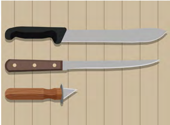
Filleting, cutting and blood knives. A short blood knife or drop knife is specially made for bleeding the fish by cutting the blood veins without damaging the meat.
