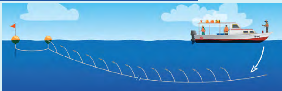
Setting a vertical longline float-first.
