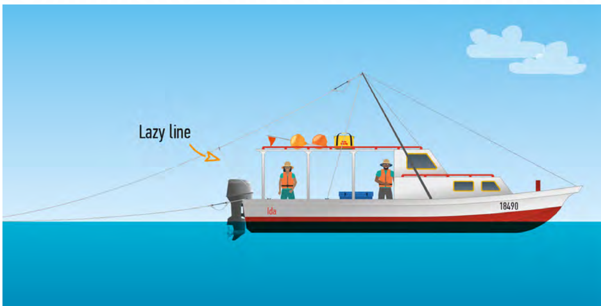
A lazy line is used to retrieve a fixed trolling line attached to the end of a boom.
