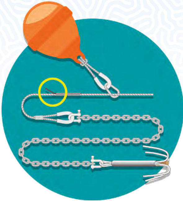
A float and non-return barb make hauling up a ground anchor much easier.
