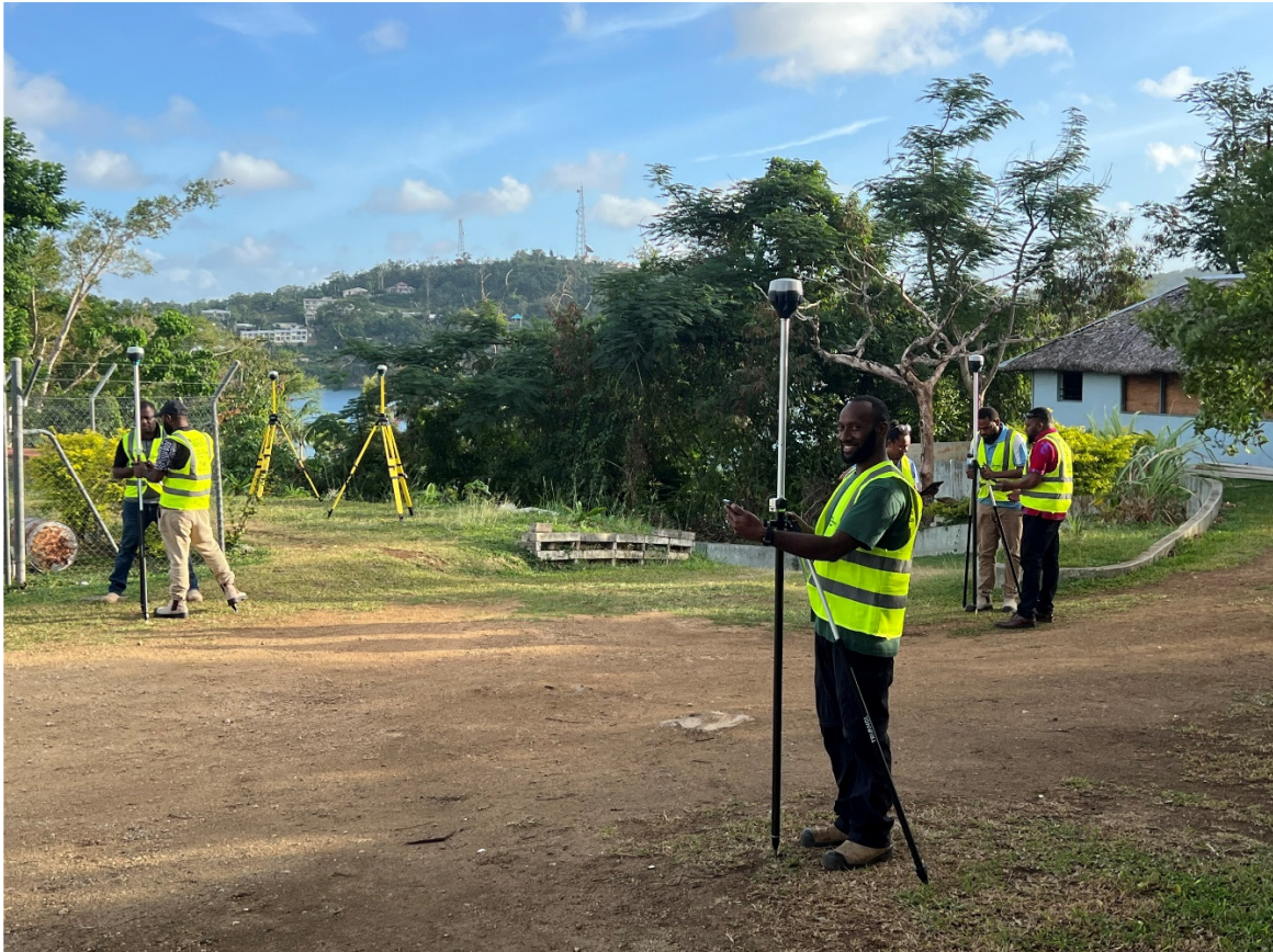
Figure 2: Trainees practising survey techniques with RTK GNSS equipment at VMGD, Port Vila
