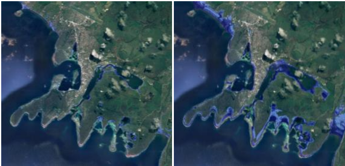
Figure 17. The Coastal Risk Dashboard allows decision-makers to explore the impacts of sea-level rise by combining climate change projections with LiDAR information into a GIS platform. (Source: http://coastalriskdb.com/ )
