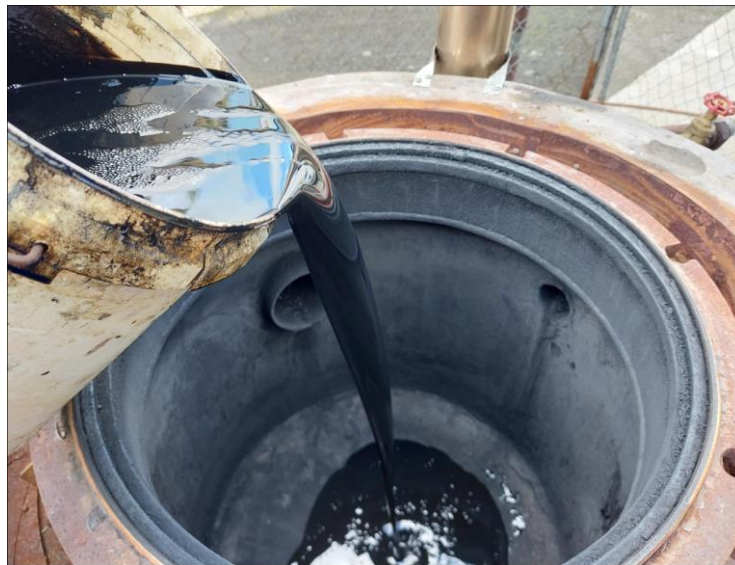
Used Oil Poured into the Pyrolysis Unit
