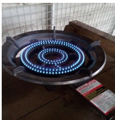
Gas hob burning gas produced
