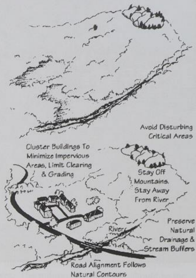
Figure 3.2 Fit the design of a site to the terrain and natural features
