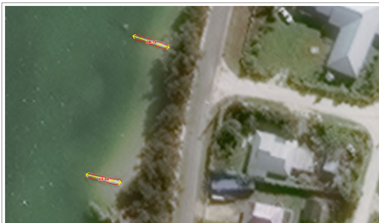
Figure 2.2.2-01: Spatial element groynes digitised with 15 cm resolution space borne image data enhanced from WorldView-3 image data of 30 cm.
