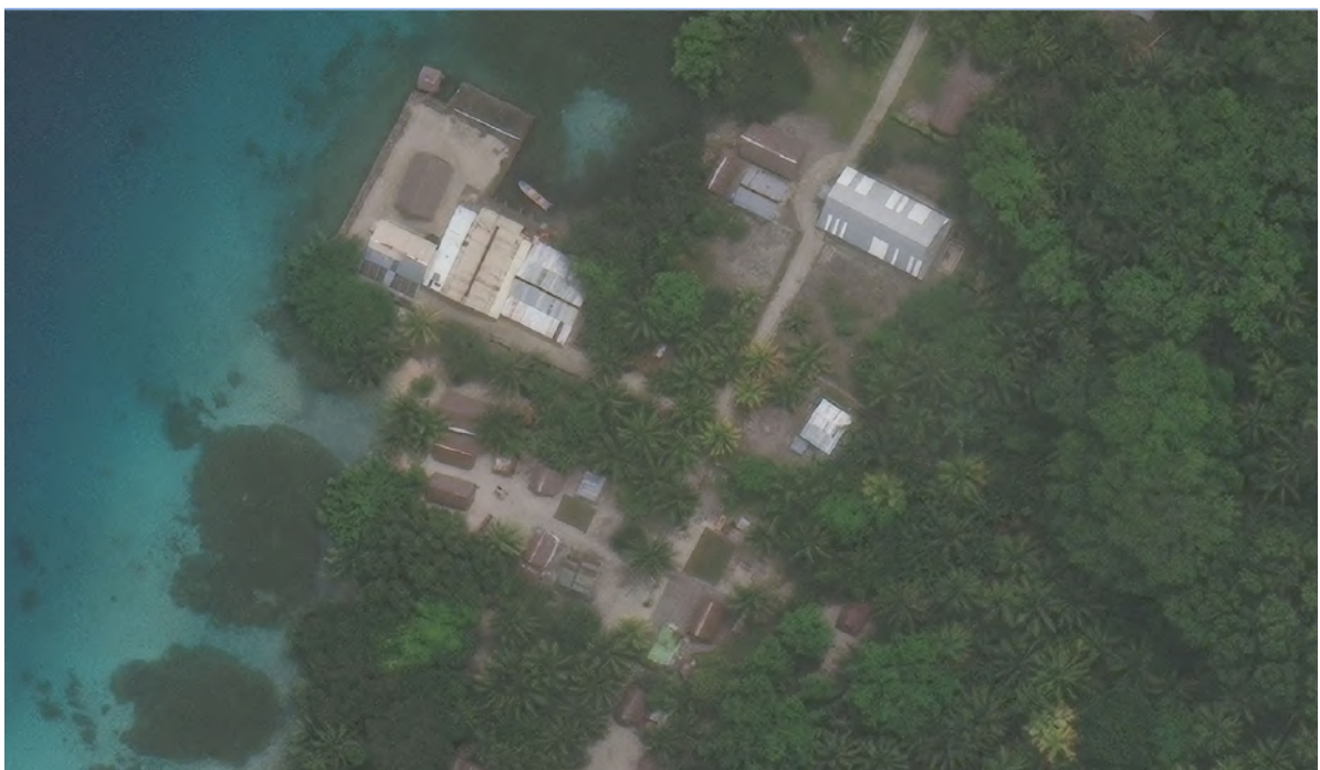
Figure 3.2.2-02: Example of metallic and pandanas covered roofs visible in the image data
