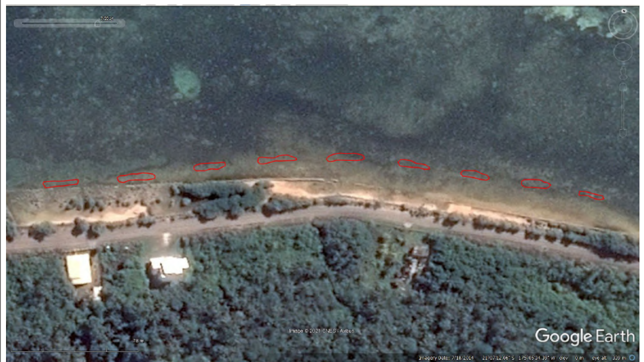
Figure 4.3-02: Location of breakwater polygons on space borne image data recorded on 18 July 2014. The detached breakwaters were not constructed yet
