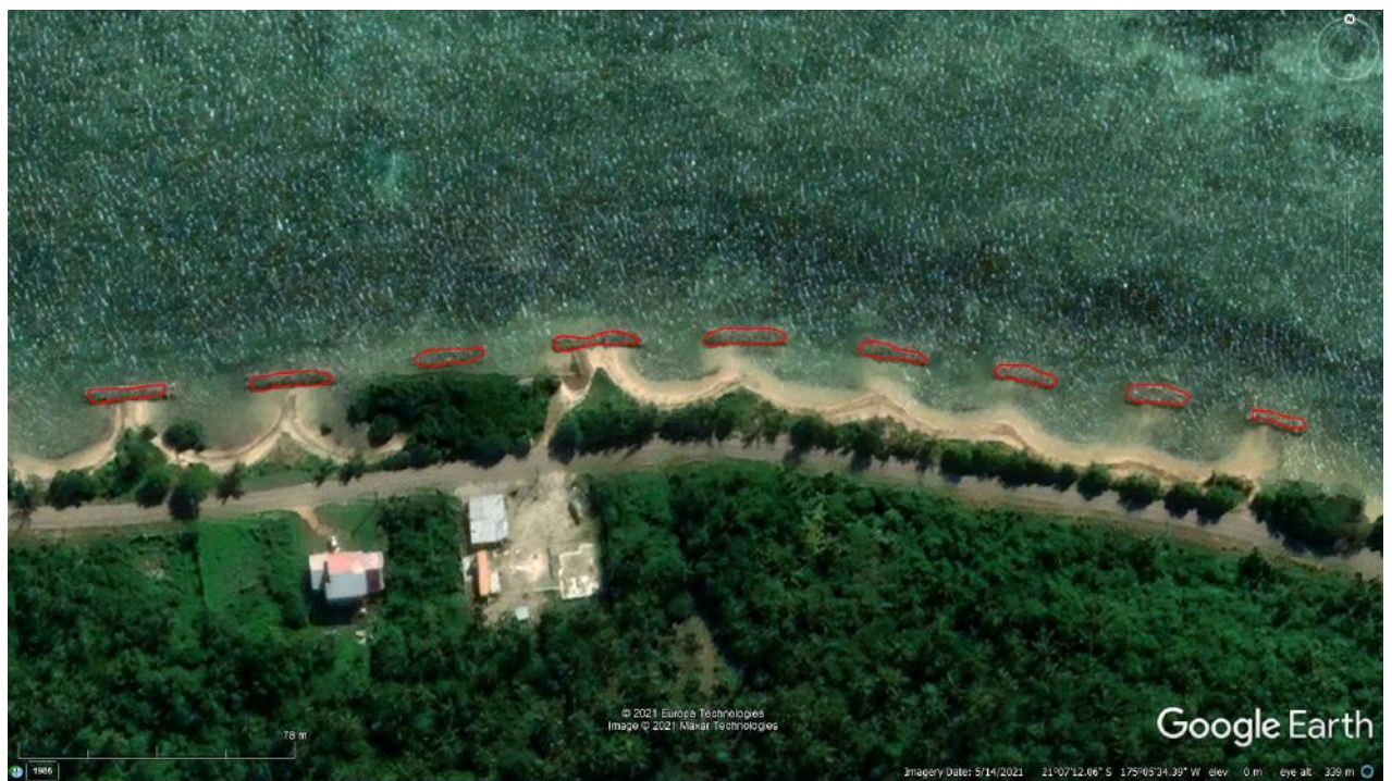
Figure 4.3-04: Location of breakwater polygons on space borne image data recorded on 14 May 2021. Vegetation is visible on the accumulated sand.
