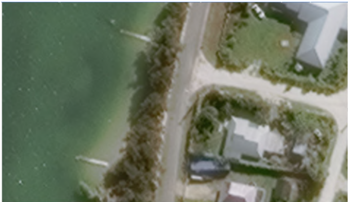
Figure 4.3.1-01: Satellite image data of 15 cm spatial resolution allow the identification of the groyne established during the last years.
