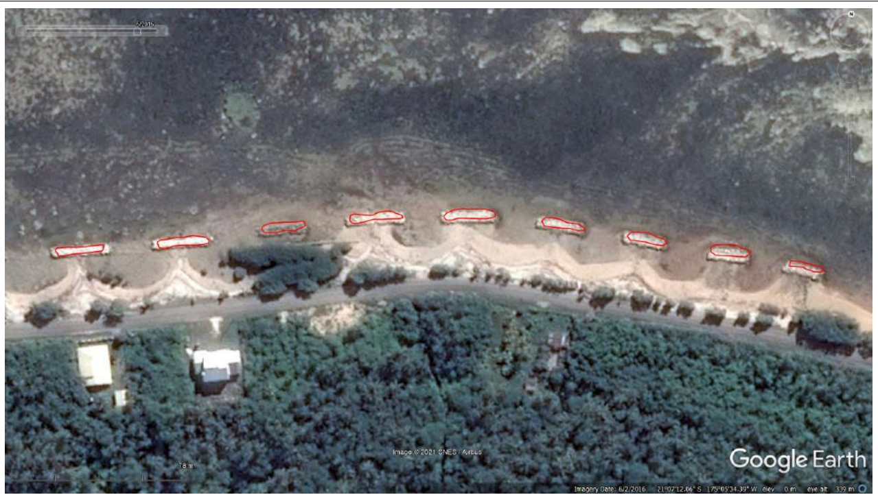
Figure 4.3-03: Location of breakwater polygons on space borne image data recorded on 02 June 2016. The breakwaters were constructed and started to change the shoreline.
