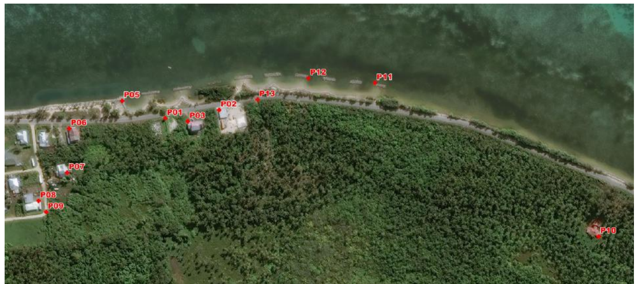
Figure 5.4-02: Image reference points distributed over the image. Important is to have points at the outer area of the image such as point 08 and point 10.
