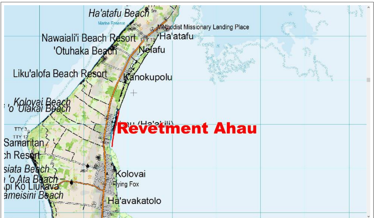
Figure 3.4-04: After digitising the revetment of Ahau on Google Earth display the line element was imported to GIS. The GIS elements allow labels (Revetment Ahau) and the calculation of the length (806 metres).
