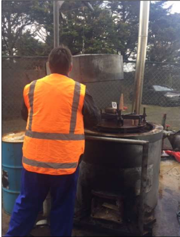
Lid Placed on Pyrolysis Unit
