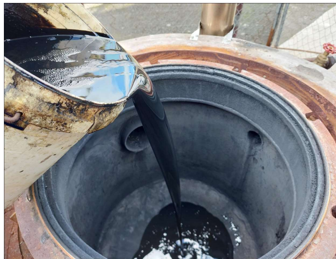
Used Oil Poured into the Pyrolysis Unit
