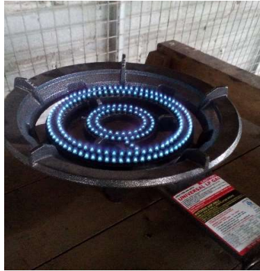
Gas hob burning gas produced
