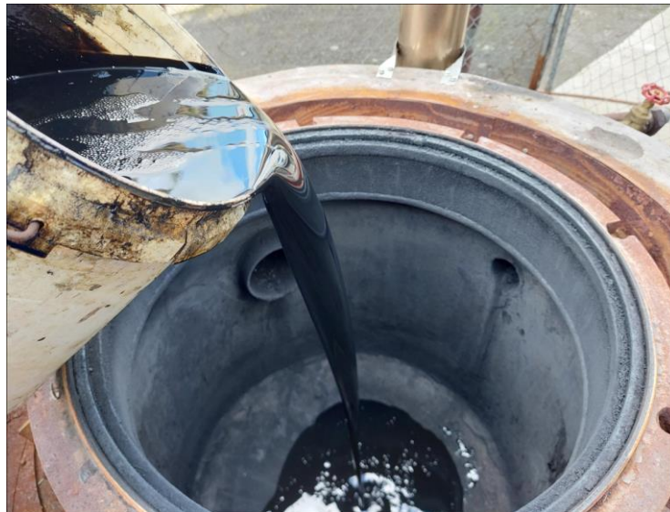
Used Oil Poured into the Pyrolysis Unit
