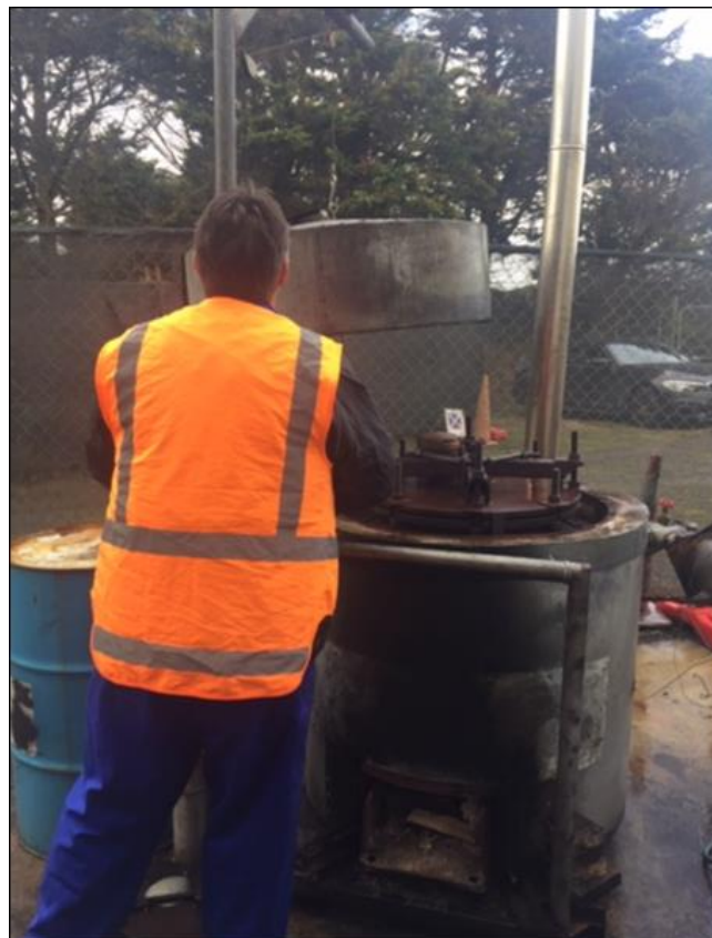
Used Oil Poured into the Pyrolysis Unit
