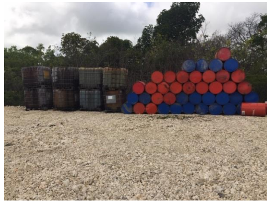
Photos 4: Drums and IBCs stored un-banded
