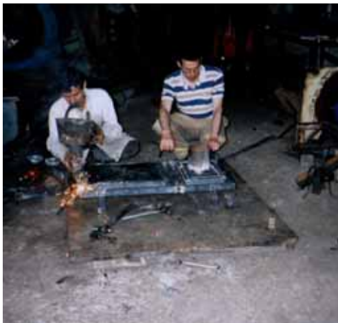
Photo 2: welding of steel top with door and chimney spigot
