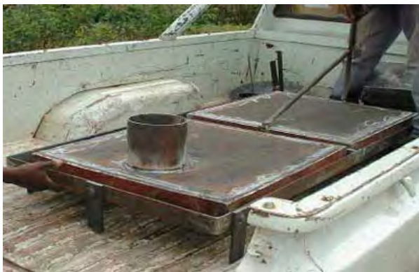
Photo 3: welded steel top with door and chimney spigot ready to be installed
