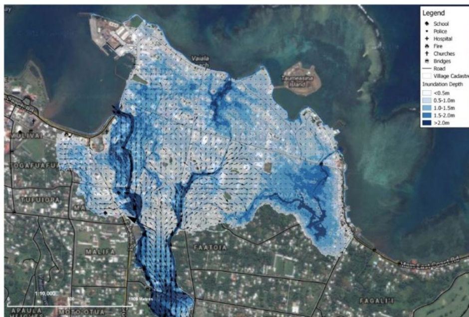
Figure 11. Flood map extent for extreme rainfall conditions obtained using a hydrodynamic model (Green Climate Fund, 2016).
