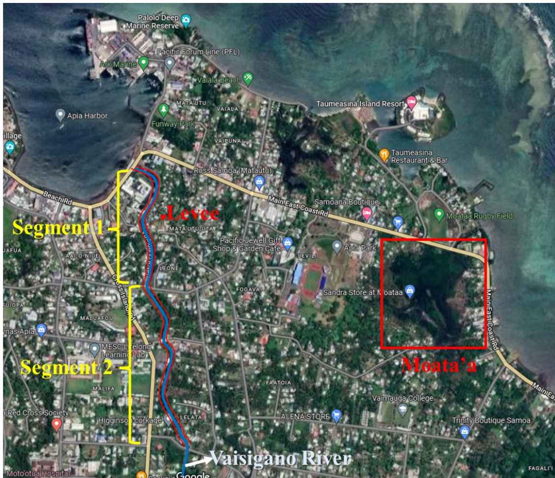
Figure 57. Levees in the Vaisigano river. Segment 1 (already constructed) and segment 2 (proposed by Filer et al. (2019)). Figure taken from Google Maps.
