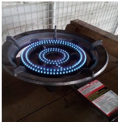
Gas hob burning gas produced
