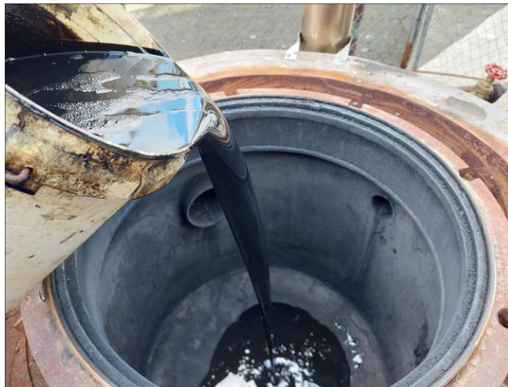
Used Oil Poured into the Pyrolysis Unit
