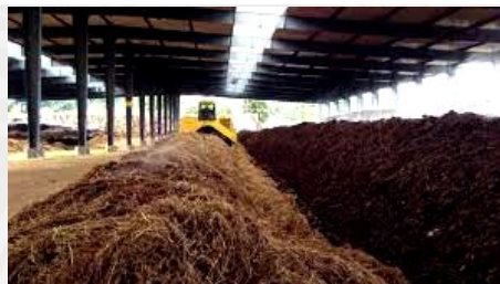
Windrow Composting – this factsheet Organic material is composted in long windrows
