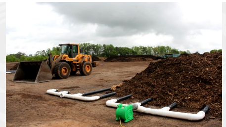
Aerated Static Pile Composting – Factsheet #8 Organic materials is composted in large piles aerated through perforated pipes
