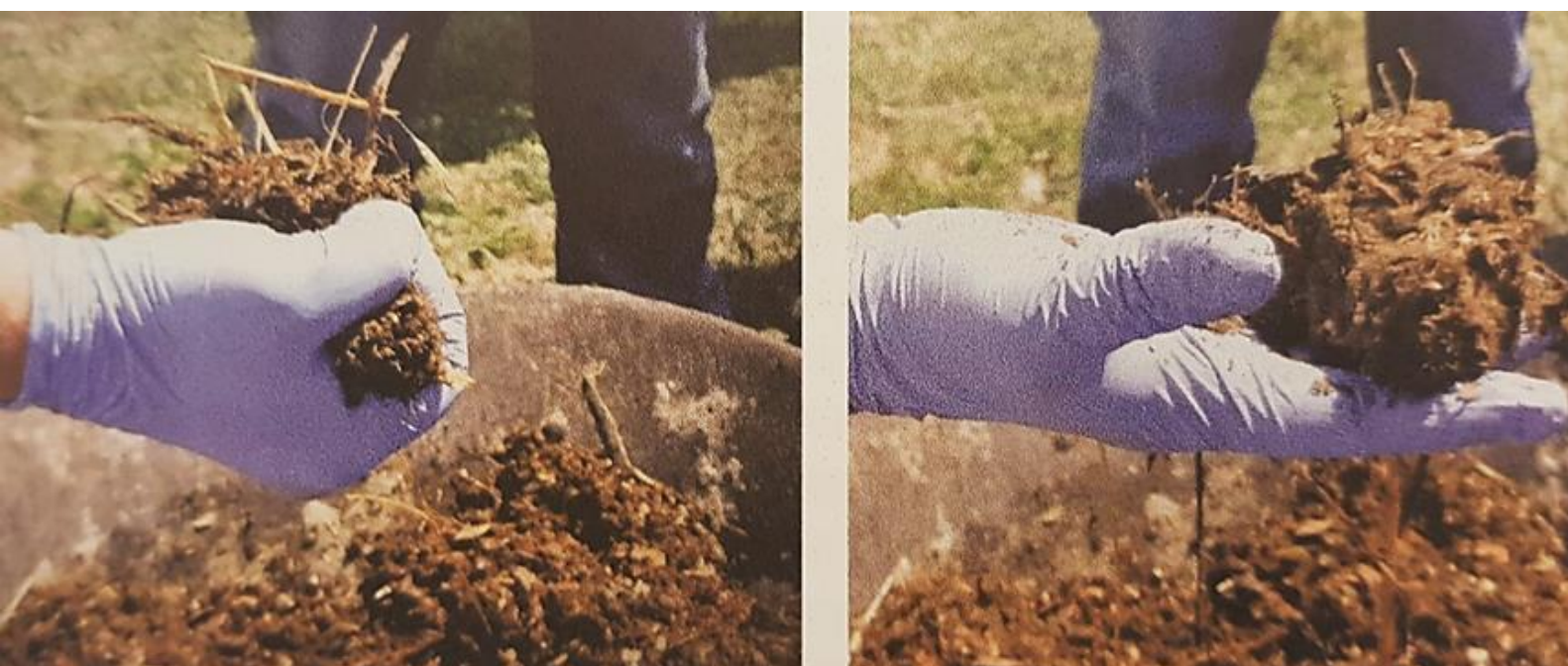
Figure 4: Example of the hand squeeze test, where the material holds together after releasing the squeeze, indicating an approximate moisture content of 50% - 55%. [Source: Rynk et al 2022]
