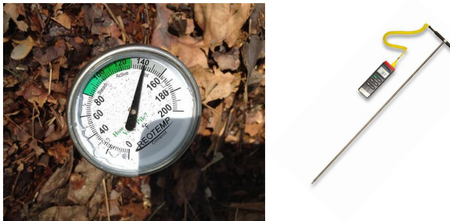
Figure 2: Temperature probes of varying length (30 – 150 cm) are available with dial readout (left) or digital display (right)
