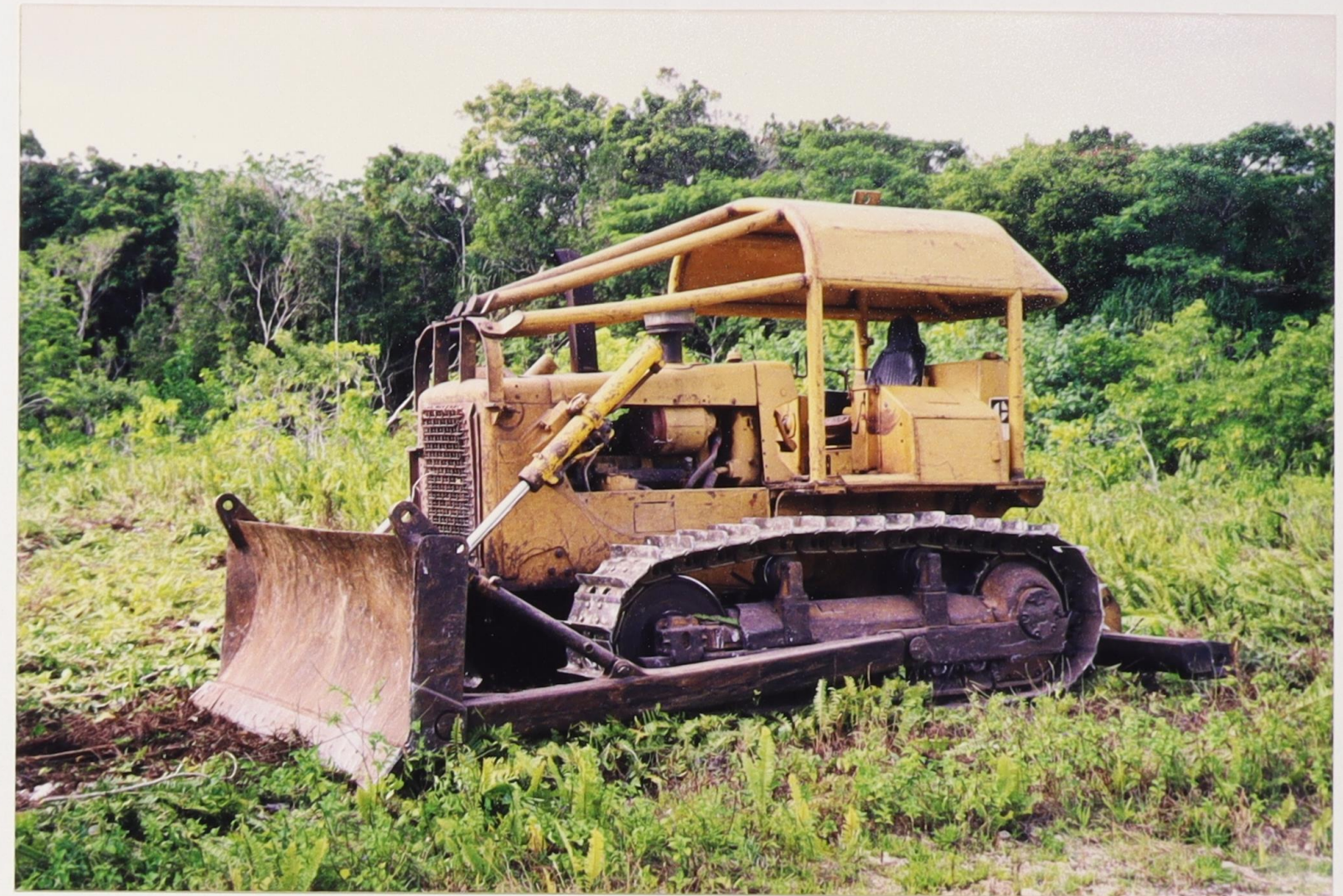
Figure 8 The main method of clearing land for agriculture in Niue is the use of bulldozers. These can clear land faster than traditional methods of land clearing. However, there are serious concerns about the environmental impact of bulldozers on the soil and on island flora and fauna.
