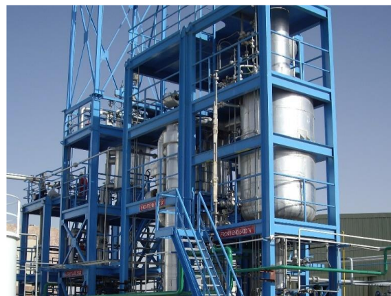
Image: used oil distillation plant (Germany)
