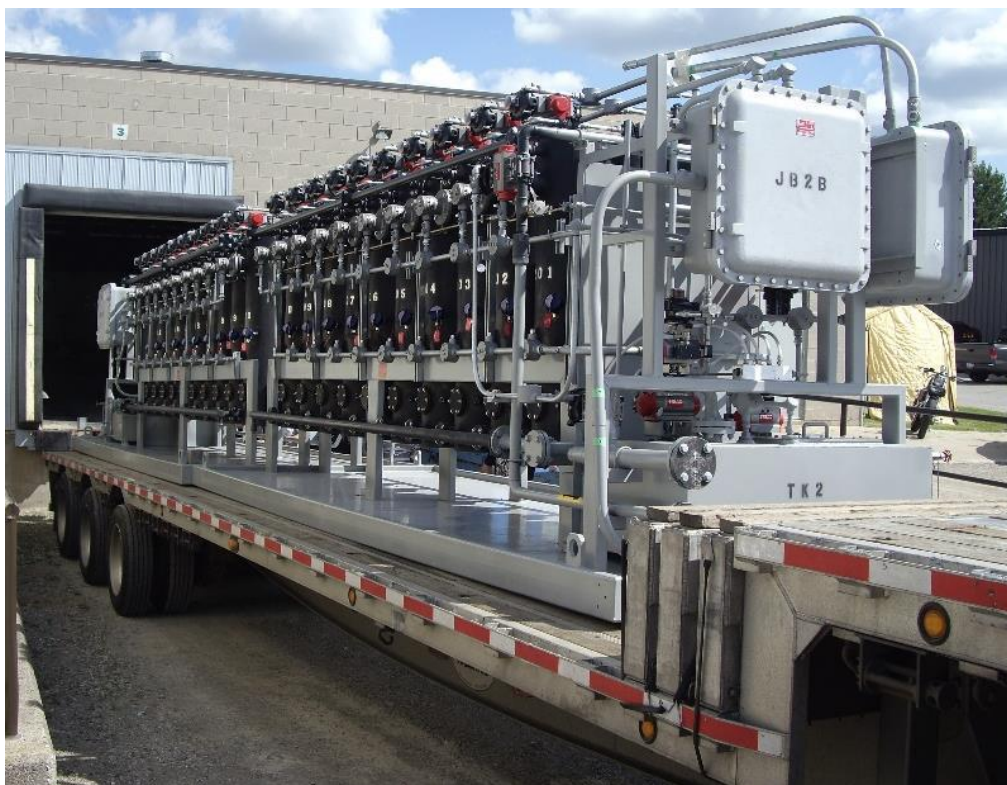
Figure 10 Transportation of back-end activated clay scrubbing unit (Germany)
