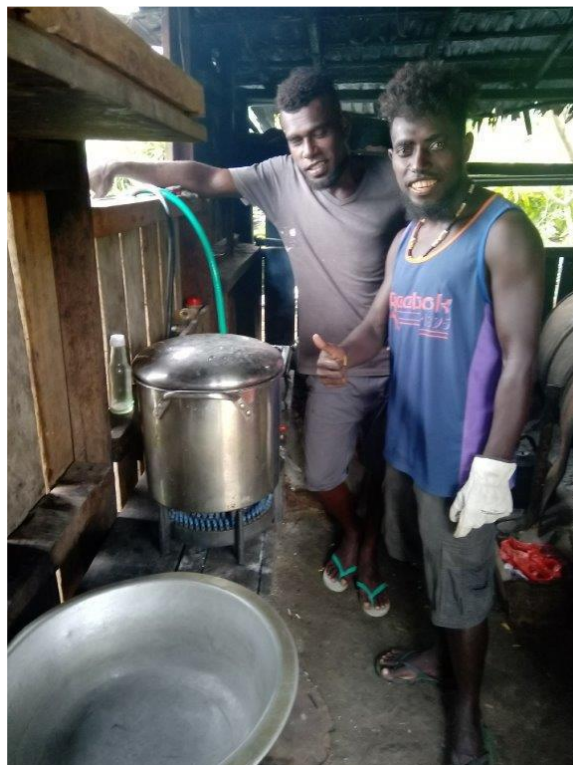
Figure 6 Direct use of pyrolysis gas oils for cooking (Solomon Islands) 34
