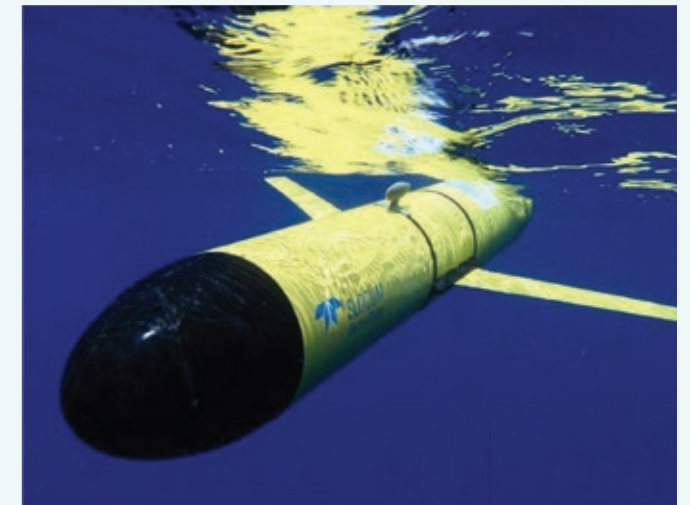
Photo: A Slocum underwater glider. Photo courtesy of Woods Hole Oceanographic Institution.
