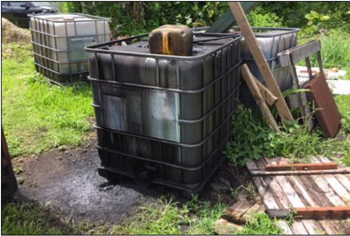
Leaking Used Oil IBCs in Niue
