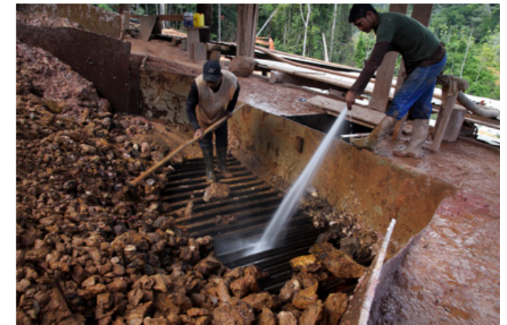
Demonstrating a new shaking table that uses only water and gravity as an alternative to the more common mercury method to extract gold from ore. Saramacca district, Suriname. Photo: Ranu Abhelakh/Reuters
