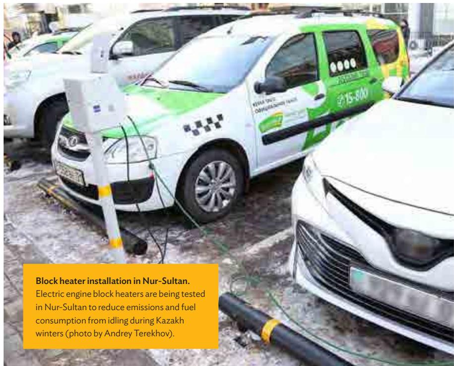
**Block heater installation in Nur-Sultan.** Electric engine block heaters are being tested in Nur-Sultan to reduce emissions and fuel consumption from idling during Kazakh winters (photo by Andrey Terekhov).
