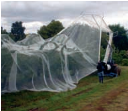
Figure 4.24: One of the net machines available that growers use to save on labour costs of netting. Photo: A. Carter.
