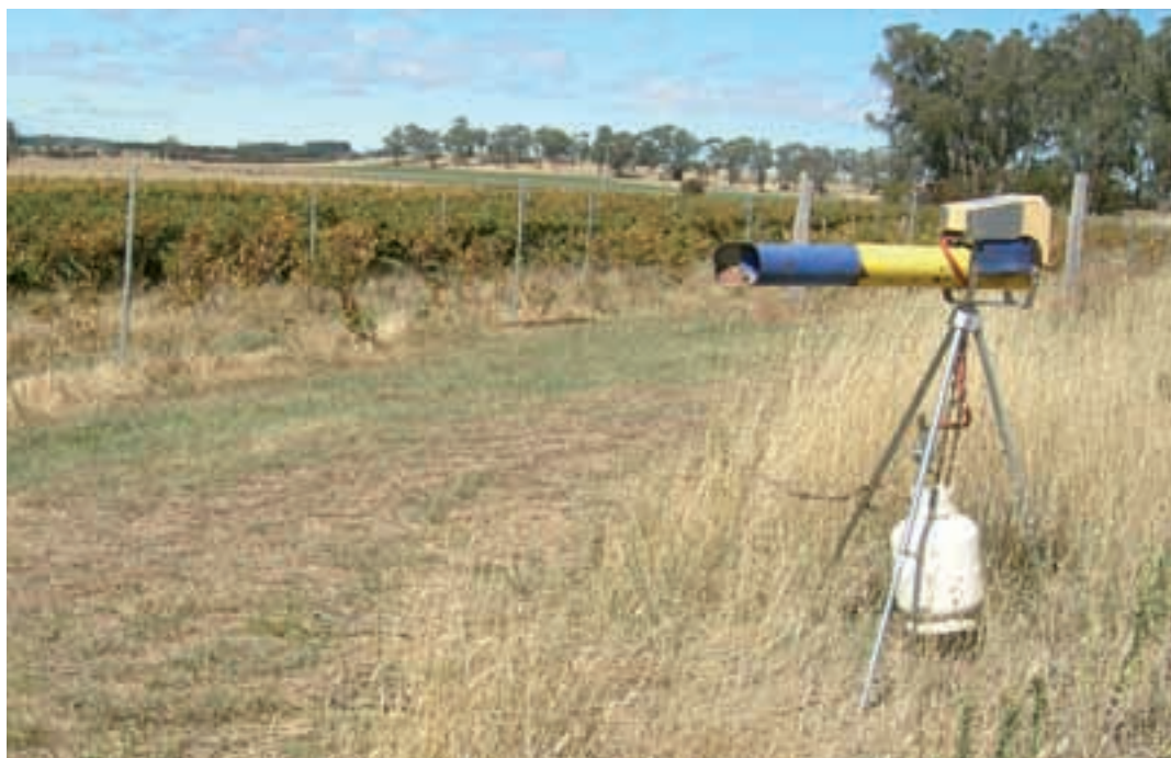
Figure 4.7: Gas gun. These devices produce loud bangs at intervals to deter birds from a crop. Note that the placement of such devices near dry grass or other flammable material poses a fire hazard. Photo: N. Reid.
