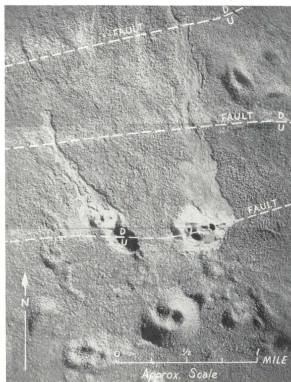
Fig. 1B: Vertical view of same area as in fig. 1A. Maugu Mu, 5,260 ft (right), and unnamed cones (left) lie on a fault scarp. The short lava flows spilled over two other fault scarps, shown by light reflected from steeper slopes and by constriction on flows. The upper scarp is some 500 ft high and extends for 10 miles from Sataua.
