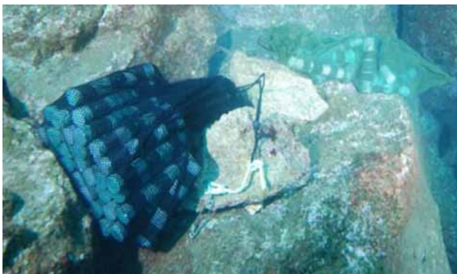
Fig. 12.4: Bags with copper sulfide “refills”.
