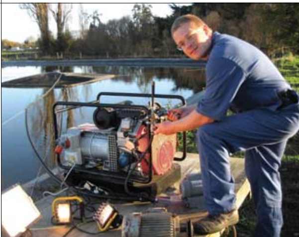
Stephan Heubeck demonstrates a generator converted to run on biogas from a dairy farm effluent pond.
