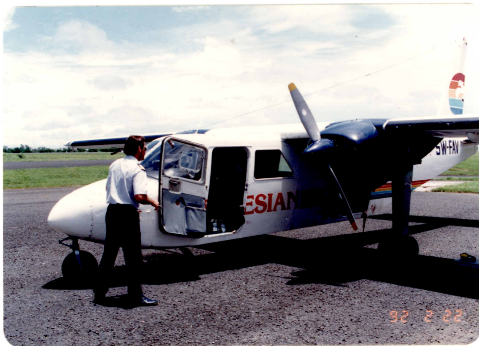
Figure 2. Britten-Norman Islander aircraft chartered from Polynesian Airlines for the air photo survey. The camera is mounted outside of the rear door of the aircraft.
