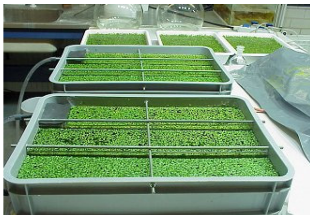
Fig. 6- Duckweed in simulated treatment plants.
