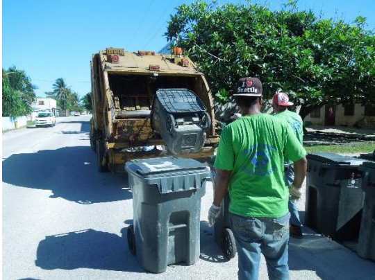
Loading of wastes from wheelie bins with loading device.
