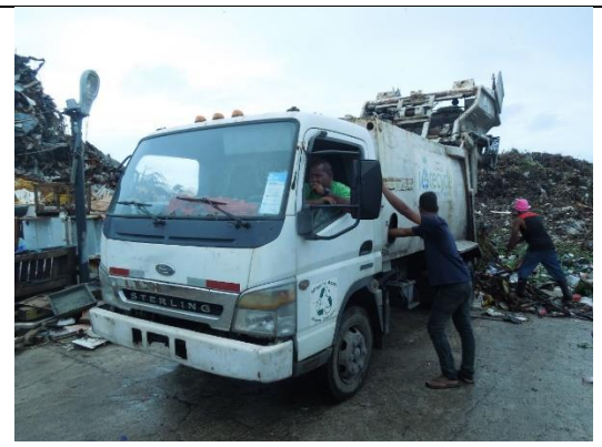
Small US made compactor truck delivered in 2009. Capacity is 4 to 6 tons(out of order as of May 2019).
