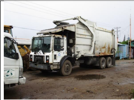
Front loading compactor truck used for transporting commercial wastes (out-of-order as of May 2019)
