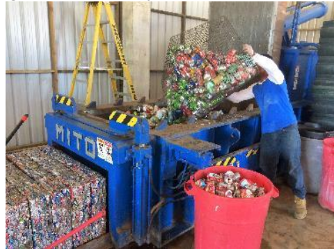
Cans are Compressed by a baling machine
