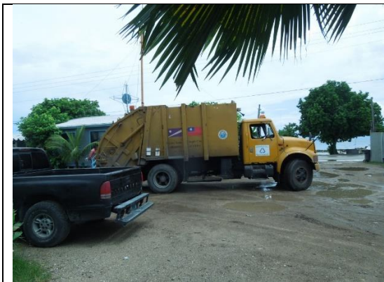
Yellow US-made compactor truck delivered in 2011 through a donation from Taiwan. Capacity is more than 8 tons (out of order as of May
