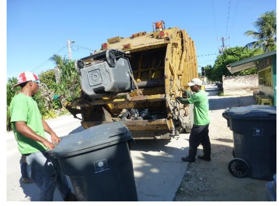
Discharging wastes from wheelie bins into compactor truck
