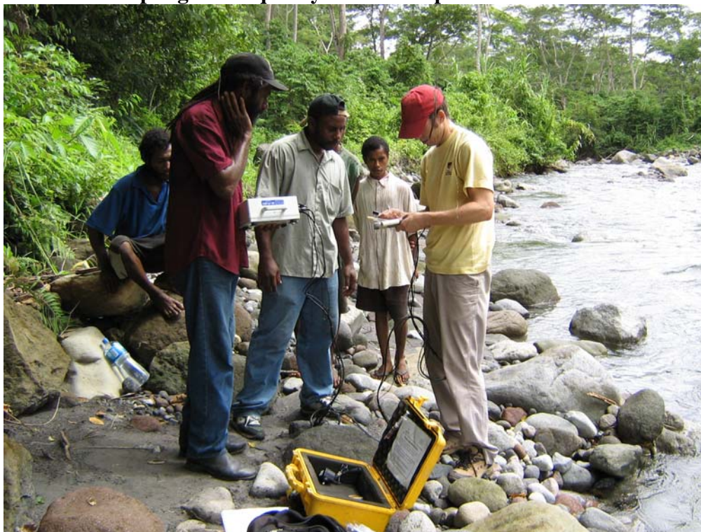
Plate 1: Sampling water quality with multi-parameter monitor.
