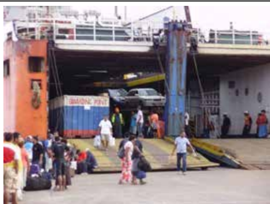
Figure 4-9 A ferry boat accommodating containers, automobiles, trucks and passengers (domestic terminal in Suva)
