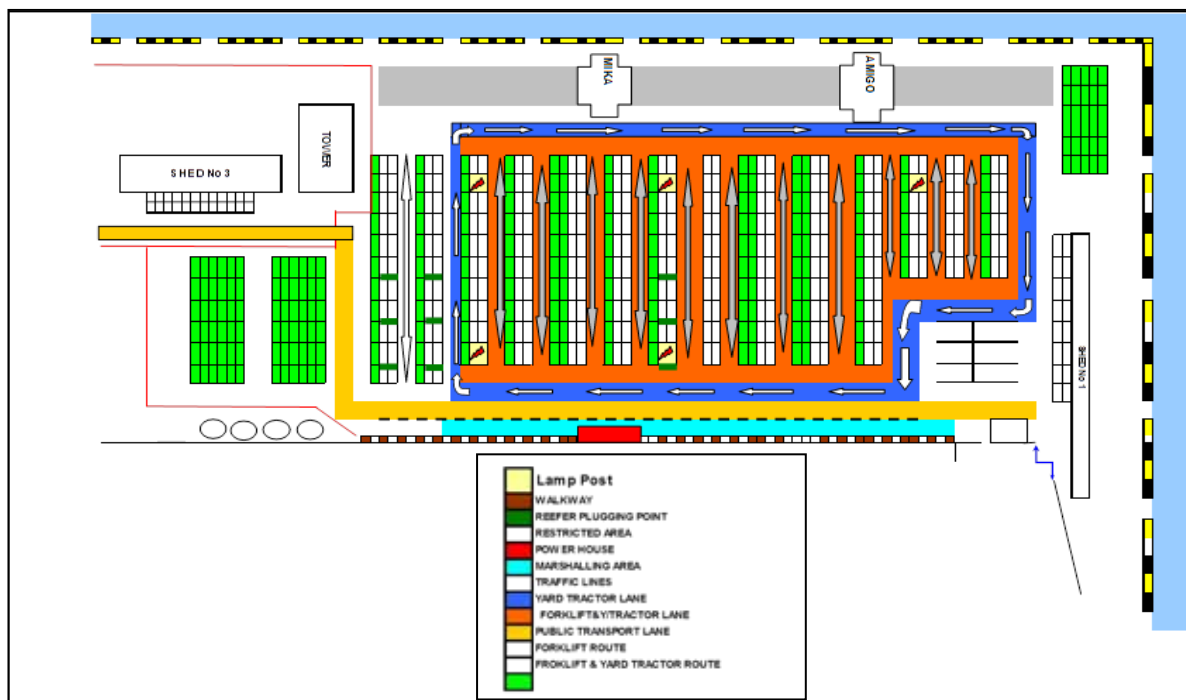
Figure 4-13 Yard layout of Suva Container Terminal
