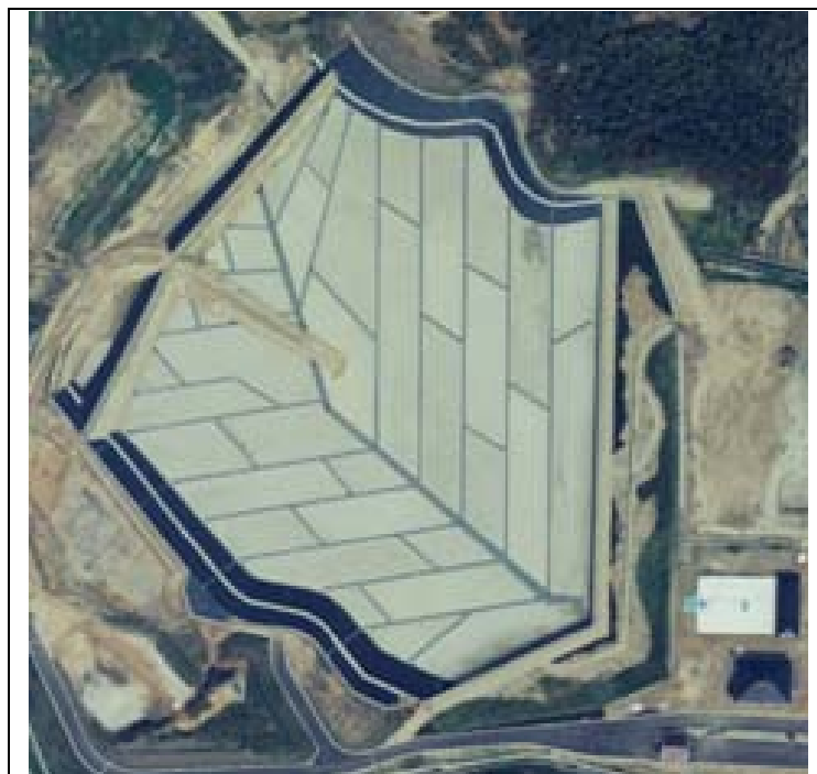
Picture 2-10 Placement example of leachate collection discharge pipes at Fukuoka-shi, Nakata Landfill
