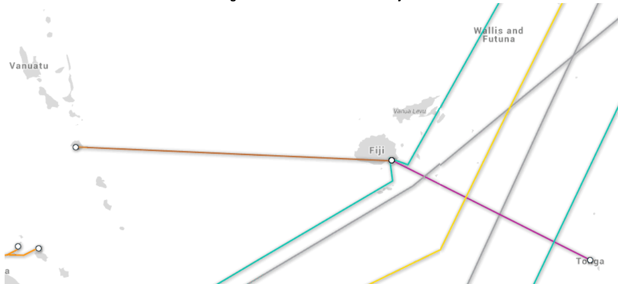
Figure 2.7: Submarine cables in Fiji
