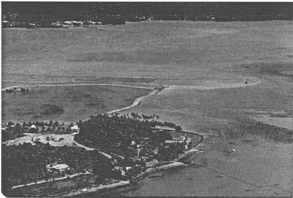
Figure AI/3. Top: a) Oblique aerial photograph of the Royal Samoan Hotel site showing the reef flat borrow pits and reclaimed land (island). The beach in the centre of the island indicates westward longshore drift as evidenced by sand buildup on the western (right) seawall. View to south. Bottom: b) Distal end of Mulinu'u Peninsula showing the nearshore dredging operations, causeways, and rock groins. Sand buildup on the groins indicates westward drift. View to south.
