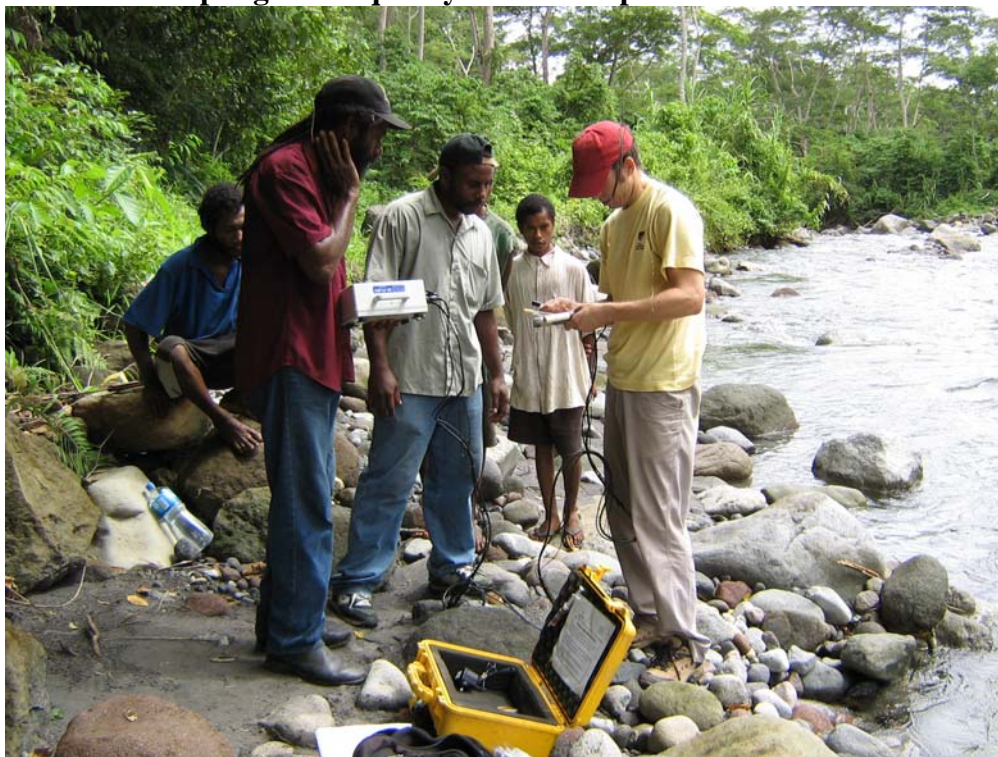
Plate 1: Sampling water quality with multi-parameter monitor.
