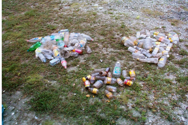
Figure 12: PET plastics content, showing (from top left) drink bottles, cooking oil bottles and other PET items
